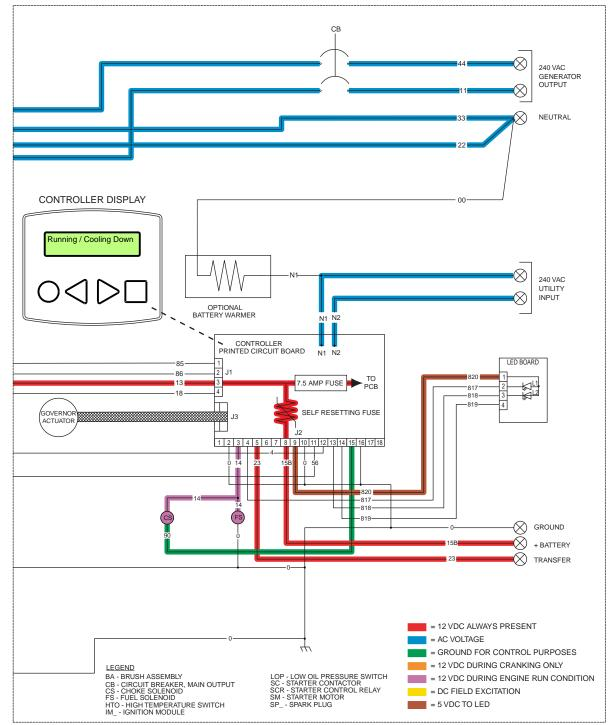
Figure 6. Circuit Condition - Utility Voltage Restored
